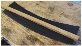
2. Wrap around a former, in this case a length of square wood and fix together with duck tape
